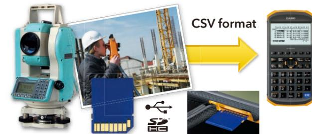
Some surveying instrument models are not equipped with USB ports or SD slots. It is possible to analyze and obtain measurement data using the programming function. Imported data in the prescribed format can be selected according to subsequent requirements from a matrix, spreadsheet, or list.
