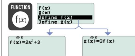
You can store functions in both the f(x) and g(x) memory. Press the (f(x)) key to display a menu for defining functions and calling the functions stored in f(x) and g(x). Call the function saved to the function memory from the different calculator apps.
