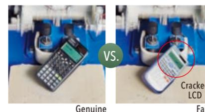
**Drop testing from a height of 75 cm**
